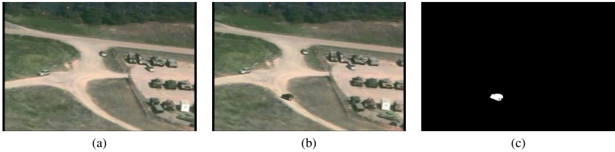
Figure 8. (a) Reference image, (b) real blurred and occluded observation, and (c) detected occlusion.
