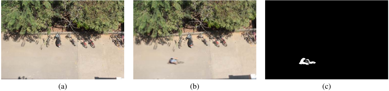
Figure 7. (a) Reference image, (b) real blurred and occluded observation, and (c) detected dynamic occluder.
