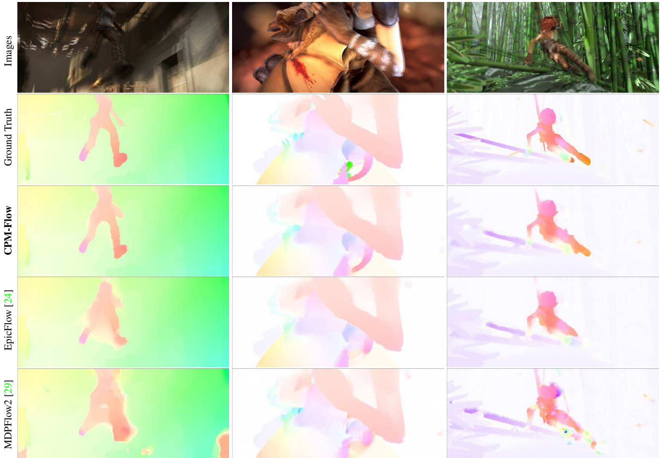
Figure 7. Example of our results on MPI-Sintel. Each column shows from top to bottom: mean of two consecutive images, ground truth, CPM-Flow and 2 state-of-the-art methods (EpicFlow [24] and MDPFlow2 [29]). CPM-Flow is able to capture thin moving objects like the tail of the monster (middle column) and the limbs of the character (right column).
