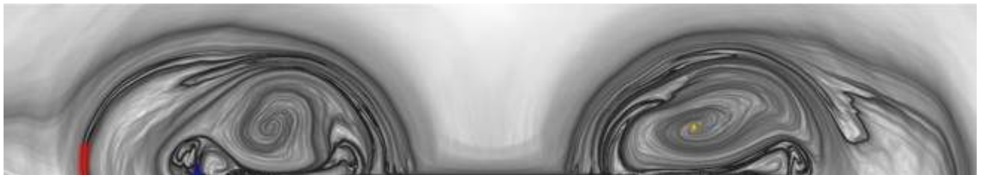
(c) Planar FTLE visualization on a section plane perpendicular to the main flow direction. Darker regions correspond to regions of high FTLE. Colored regions indicate PDFs that were used to seed pathlines for (b).
