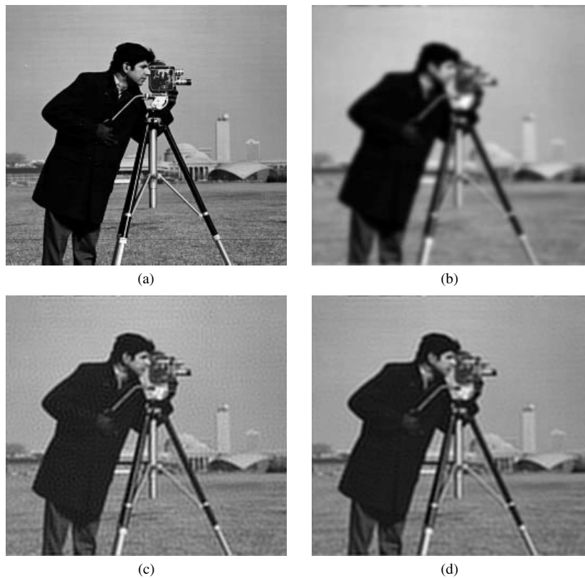
Figure 10. (a) Original cameraman image. (b) Blurred, noisy cameraman image. (c) Restored by using the regularization parameters minimizing the MSE. (d) Restored by using the regularization parameters obtained by our iterative algorithm.
