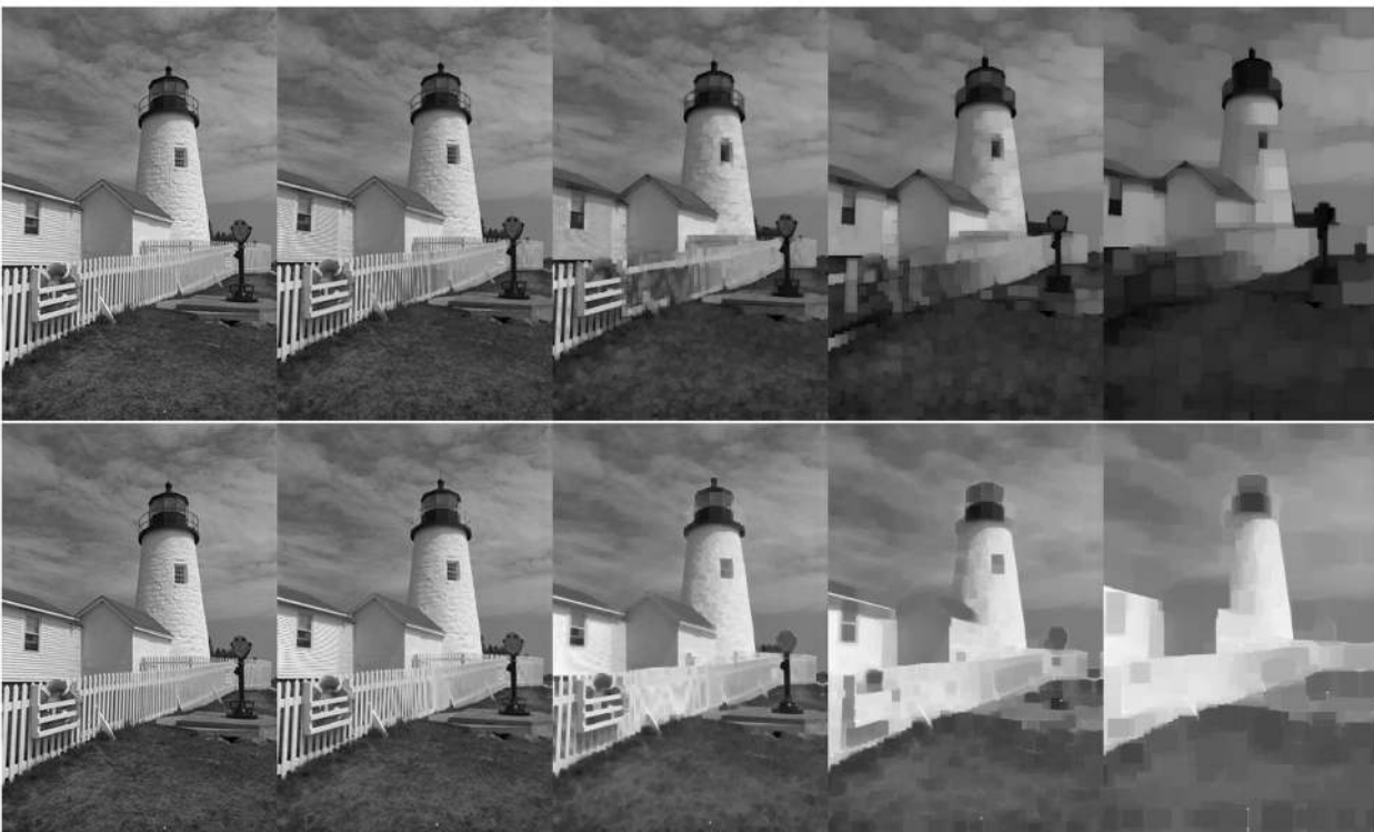
Fig. 2. The effect of the opening (top) and closing (bottom) filters. (Original image is shown on left frame, followed by the filtered image using rectangular windows sized 2 \times 2 , 4 \times 4 , 8 \times 8 , and 16 \times 16 .)
