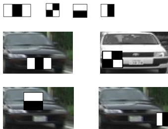
Fig. 3. Haar-like feature examples for describing a vehicle's appearance.
