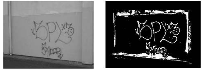
Figure 4: Image binarization. Left: image after pre-processing; right: image after binarization
