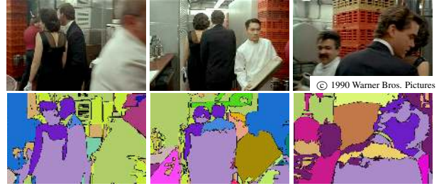
Figure 4: Clip-based processing, optical flow edges and region features for segmenting long video clips (28 s) from Goodfellas, ©1990 Warner Bros. Region identity of the actors is preserved under partial occlusions, motion blur and complex background.
