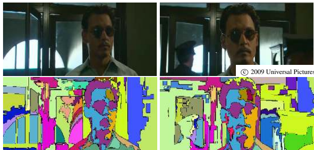
Figure 11: Failure case. Encoding artifacts cause fragmentation (wall on the right). The algorithm can be sensitive to smooth illumination changes (background) and hard shadows (on the face). Original frame from Public Enemies , ©2009 Universal Pictures.
