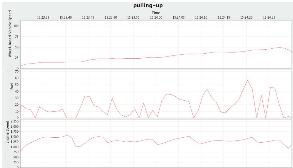
Figure 6.8: A typical example of the sensor values when a truck pulls-up (normally) from 0 to 50 km/h.
