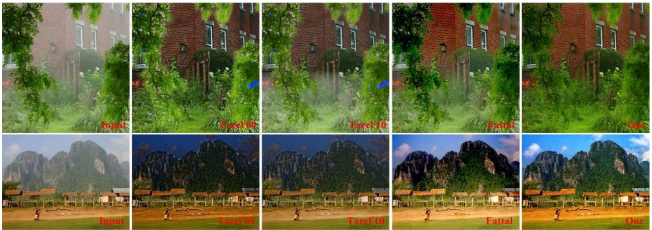
Figure 8. Comparisons with Tarel et al. 's method and Fattal's method. From left to right: input haze images, the results of Tarel et al. 's method in ICCV'09, the results of Tarel et al. 's method in IV'10, Fattal's results, and our results, respectively. (Best viewed in color)
