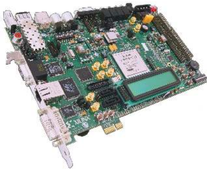
Fig. 1. Picture of a Virtex-5 OpenSPARC Platform used for the implementation of the C-Mantec algorithm.
