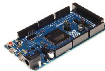
Fig. 6. Picture of an Arduino DUE board used for the implementation of the C-Mantec algorithm.
