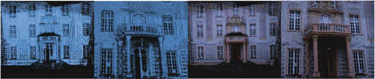
Fig. 13 Entry-P10 The 3D point cloud was constructed in 1.6 min from 10 6 Megapixel images and contains 1.4 million points. The left images The raw points and the right images The colorized versions of these points (color figure online)
