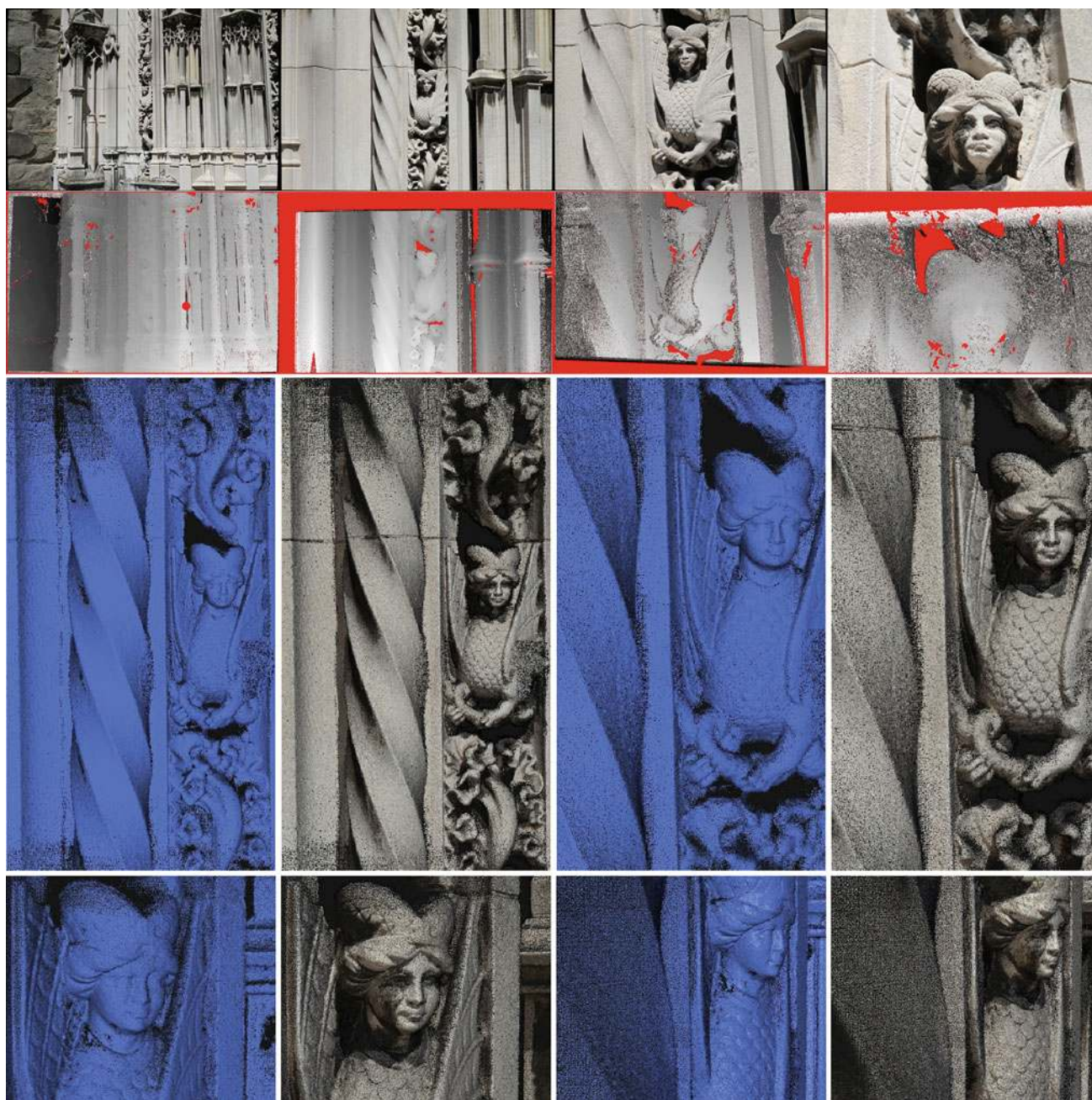
Fig. 1 Statue reconstruction. The data set contains 127 18-Megapixel images of a statue. The reconstruction time was 29.5 min and the final cloud contains 15.3 million points. First row Some images from the
