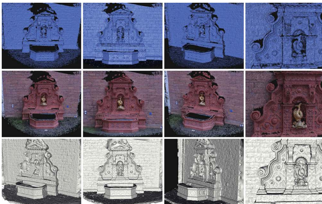
Fig. 9 Fountain-P11. The 3D point cloud was reconstructed in 2.2 min from 11 6-Megapixel images and contains 2.5 million points. First two rows The raw 3D points and their colored versions. Last row The mesh computed from these points using the Poisson reconstruction algorithm (color figure online)
