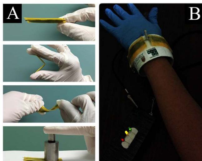
Figure 8. (A) ES cell: as fabricated and under bending, twisting and partially compressing stress, (B) wearable cells which are connected in series are able to power LED bulbs.
