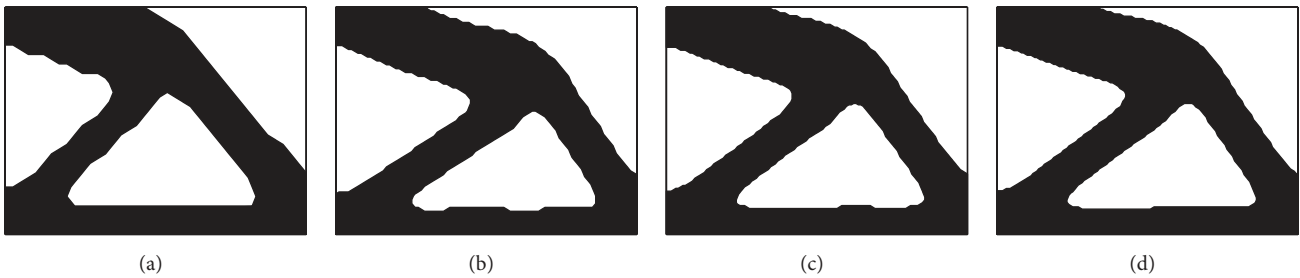
FIGURE 10: Mesh-independent solutions of the second cantilever beam: (a) 40 \times 25 ; (b) 96 \times 60 ; (c) 128 \times 80 ; (d) 160 \times 100 .
