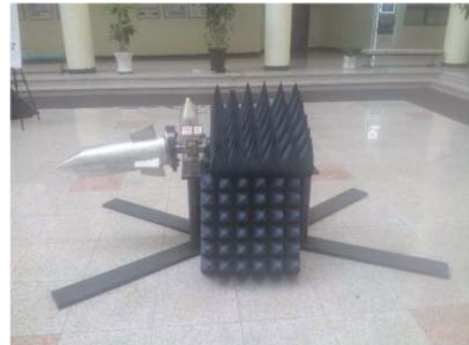
Fig. 5. Measurement setup. To eliminate the effect of micro-motion of the second motor, it is covered with radar-absorbing material.
