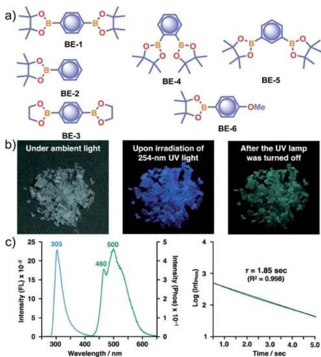
Fig. 2 (a) Chemical structure of aryl boronic esters **BE-1-6**. (b) Photographs of **BE-1** under ambient light (left) and irradiation with 254 nm UV light in the dark (middle), and after the UV light was turned off in the dark (right). (c) Fluorescence and phosphorescence spectra (left) and the corresponding phosphorescence decay profile of **BE-1** (right). Reproduced with permission from ref. 78. Copyright 2017, American Chemical Society.
