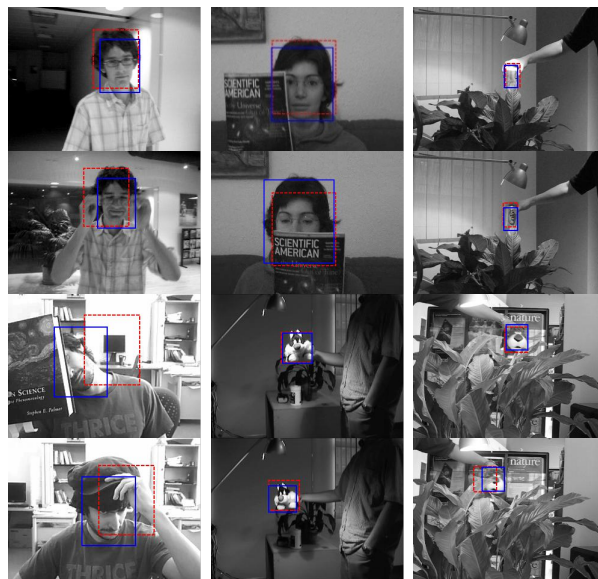
Figure 7. Snapshots of some tracking results: our tracking-by-identification method (blue) is often competitive with the more complex MILBoost algorithm of [7] (red).
