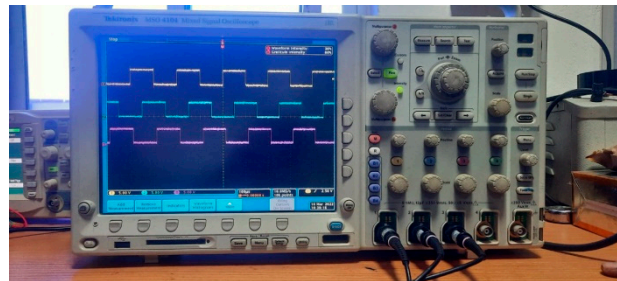
Figure 17. Pulse waveform MPIBC (six phase).
