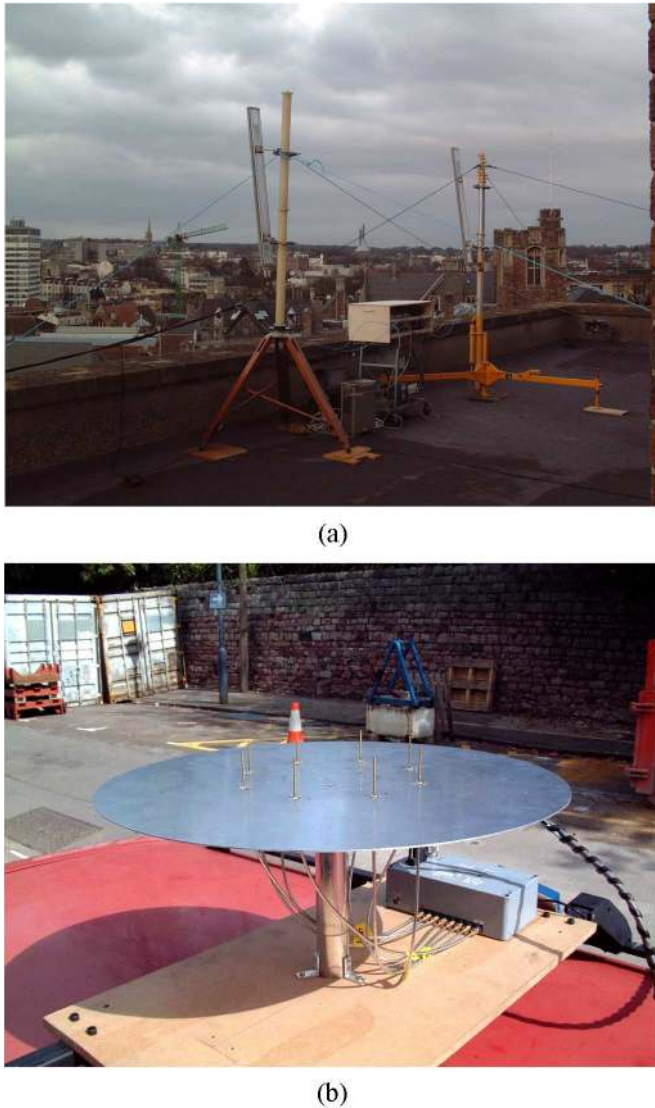
Fig. 6. (a) Transmitter mounted on building top. (b) UCA receiver mounted on car top.
