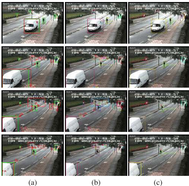
Fig. 6. Comparison of tracking results between the multi-target tracker with (PHD-MT) and without (MT) PHD filter. (a) Detections (color-coded in red) and PHD output (color-coded in green). Several false detections are filtered by the PHD (second, third and fourth row). (b) MT results. (c) PHD-MT results. False tracks due to clutter are removed by PHD-MT.
