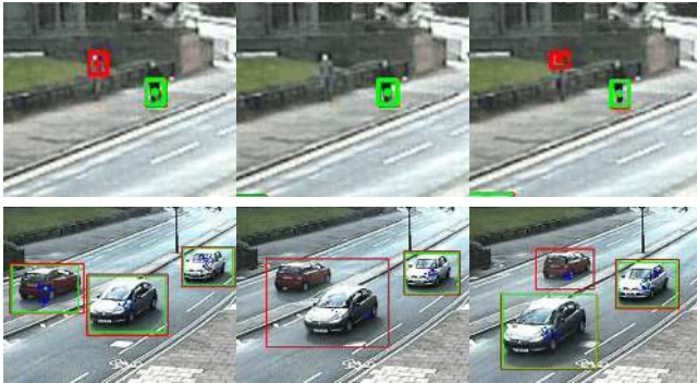
Fig. 9. Failure modalities of the Particle-PHD filter when using a change detector. The red boxes are the observations and the green boxes are the output of the PHD filter. (Top row) Inconsistent detections in the far field are interpreted by the PHD filter as clutter and therefore removed. (Bottom row) Interaction between targets (object merging) generates a bounding box for a group of objects.
