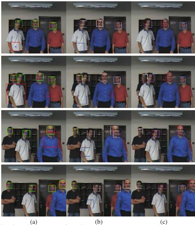
Fig. 8. Comparison of tracking results between the multi-target tracker with (PHD-MT) and without (MT) Particle PHD filtering. (a) Detections (color-coded in red) and PHD output (color-coded in green). Several false detections are filtered by the PHD (First, second and third row). (b) MT results. (c) PHD-MT results. The PHD-MT successfully recovers the faces after a total occlusion without generating false tracks.
