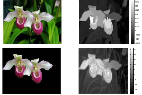
Figure 3. The region detection and segmentation algorithm. Top: Input image and the initial regions which are classified with high score to belong to either a flower or the background. Bottom: Label propagation on this image and the final segmentation result.
