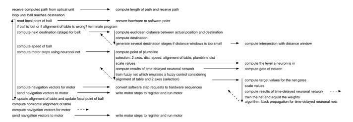
Figure 7: Functional decomposition of WobbleTable software
