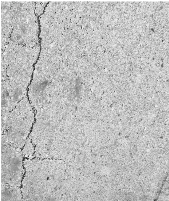
Fig. 4 Result of applying the logarithmic transform to Fig. 3. This image shows imperceptible dark details of the original image to appear more clearly
