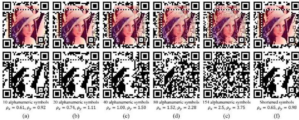
Fig. 13. QR code results generated by embedding messages of different lengths. (a)–(e) are the results of embedding 10, 20, 40, 80, and 154 alphanumeric symbols, respectively. (f) The result of embedding a shortened URL for a message with 154 alphanumeric symbols. Top and bottom rows represent the beautified QR code results and the baseline QR codes, respectively.
