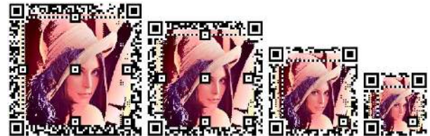
Fig. 9. QR codes generated by our method with different version number ( V = 11, 9, 6, \text{ and } 3 ).
