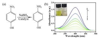
**Figure 2.** Catalytic reaction of 4-NP to 4-AP. (**a**) The catalytic reaction equation. (**b**) Time-dependent UV–Vis spectra showing gradual reduction of 4-NP over the sample Ag/p-ZnO collected in the cuvette under natural light, with digital photos of color changes before (left) and after (right) the reaction inserted.
