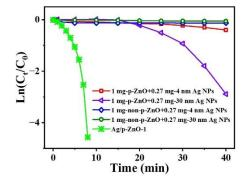
**Figure 6.** Plots of  $Ln(C_t/C_0)$  versus the reaction time for the reduction of 4-NP over different catalysts under natural light.
