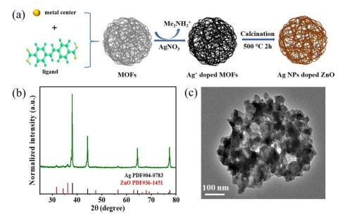
**Figure 1.** Ag-doped porous ZnO. (a) The synthesis procedures of Ag<sup>+</sup> doped MOFs via cation exchange and Ag/p-ZnO heterostructure by calcining. (b) XRD patterns of Ag/p-ZnO. (c) TEM image of sample Ag/p-ZnO.
