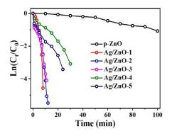
**Figure 5.** Plots of  $Ln(C_t/C_0)$  versus the reaction time for the reduction of 4-NP over the Ag/p-ZnO heterostructure under natural light.
