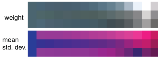
Figure 3: The complete BRDF data for the green-metallic-paint measured BRDF, using a K -term Gaussian approximation and an elevation sampling of N views. The data (means, standard deviations, weights) is stored as two texture maps of size K \times N texels. Typically we use K=3 Gaussians and N=15 views.
