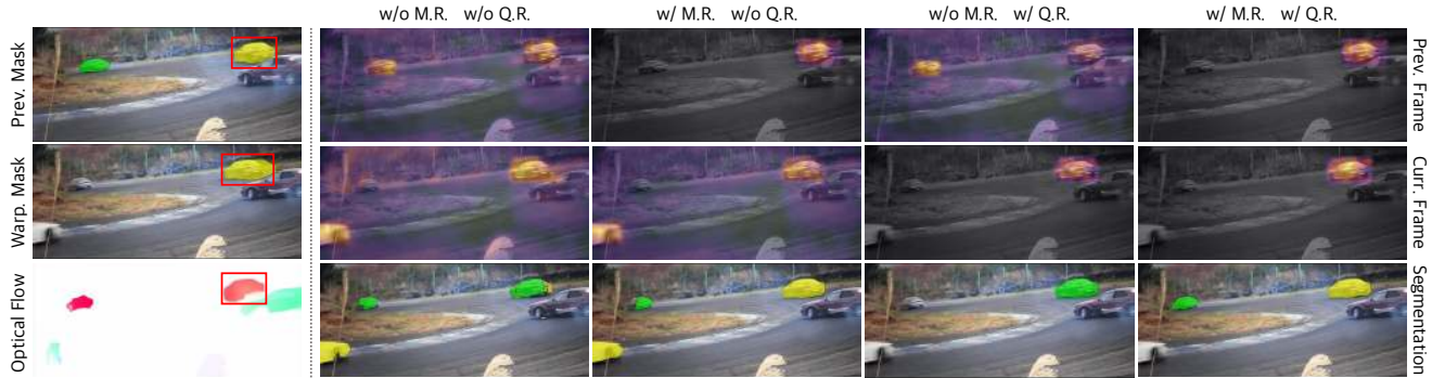
Figure 7. The similarity scores of the target object in the previous and current frames. The target object is highlighted by a red bounding box. “M.R.” and “Q.R.” denote for “Memory Region” and “Query Region” in the regional memory and query embedding, respectively.
