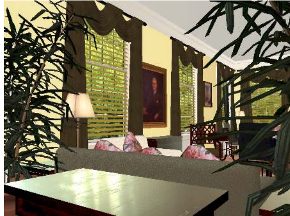
Figure 3: Software rendering simulating our prefiltered environment map technique. Specular exponents range from 1 to 5 for the couch, 5 to 15 for the grain of the wood, and 75 to 150 for the wood foreground. The wood is increasingly reflective at grazing angles.
