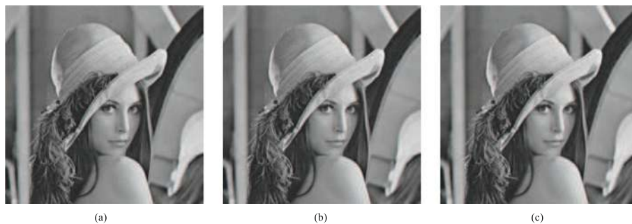
Fig. 6 Embedding distortion (in PSNR) with two group selection methods. a Lena. b Embedding 40,960 bits with Method 1 (44.914 dB). c Embedding 4960 bits with Method 2 (41.754 dB)
