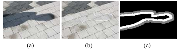
Figure 6: Shadow boundaries processing. (a) Input image, (b) shadow boundaries needed to be processed, (c) the narrow bands built around the shadow boundaries.
