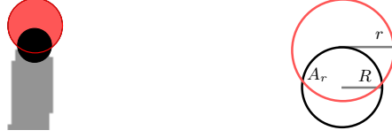
Fig. 4. Curvature calculation. The curvature at any point along the curve can be estimated from the intersection A_r of a ball with radius r centered at the curve point with the interior of the shape. R = \frac{1}{\kappa} is the radius of the osculating curve (cf. (3)).
