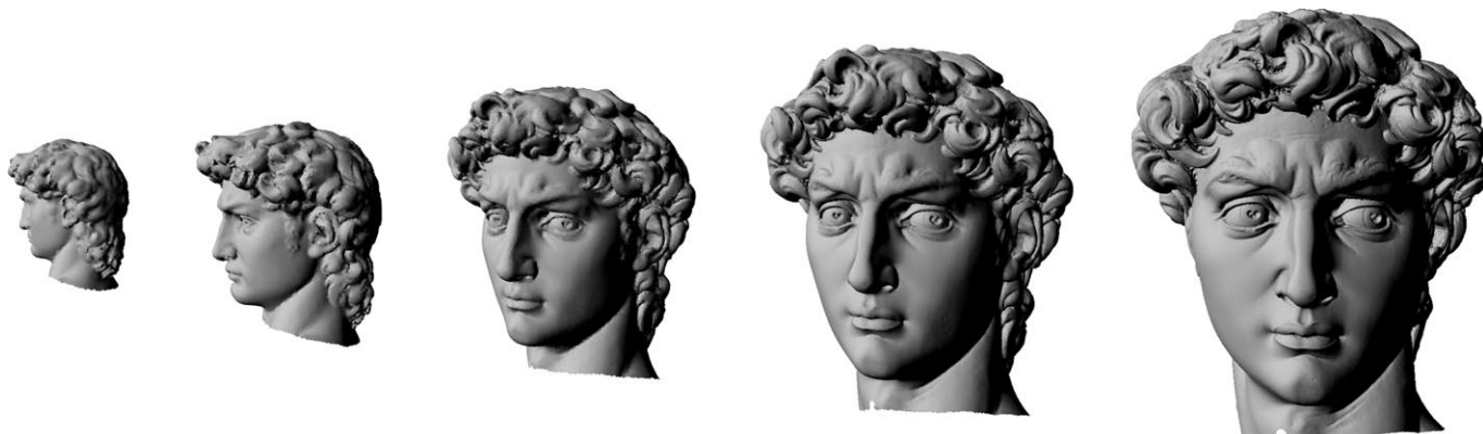
Figure 1: Michelangelo's David at different levels-of-detail. From left to right, 10k, 20k, 60k, 200k and 2000k points for the original model, rendered with a point splatting renderer.
