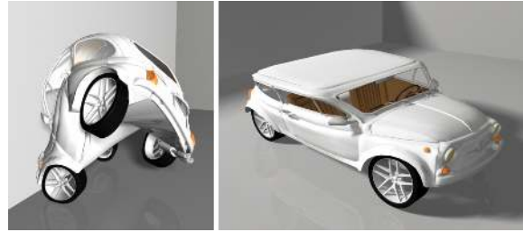
Figure 5: The elastic and plastic deformation behaviors are independently controlled for this simulated car.
