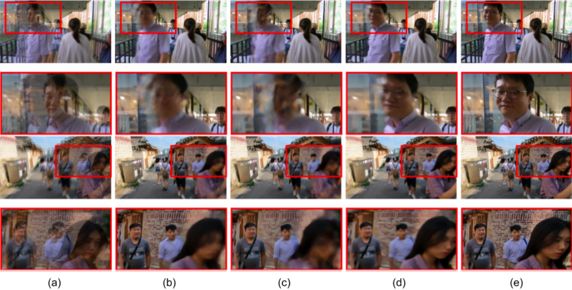
Figure 5. Comparison with state-of-the-art on Odd Frame generation. From Left: (a) Upsampled and overlaid LR frames (b) STARnet (c) Zooming Slomo (d) Ours (e) Ground Truth. Zoom in for details.
