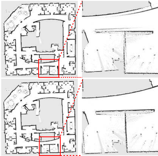
Fig. 3. Effect of the \chi^2 reduction. This figure shows two maps generated from two graphs having a different \chi^2 error. The error of the graph associated to the top map is 10 times bigger than the one on the bottom. Whereas the overall structure appears consistent in both cases, the details in the map with the lower \chi^2 appear significantly more consistent.
