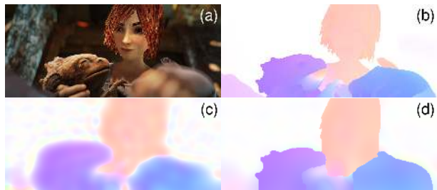
Figure 5: Results on MPI-Sintel: (a) Image; (b) Ground truth flow; (c) PCA-Flow; (d) PCA-Layers.
