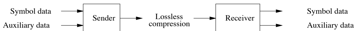
FIGURE 2. A scheme in which auxiliary data is communicated along with the primary symbol data in order to achieve optimal compression when the source code produces multiple codewords for a given symbol.
