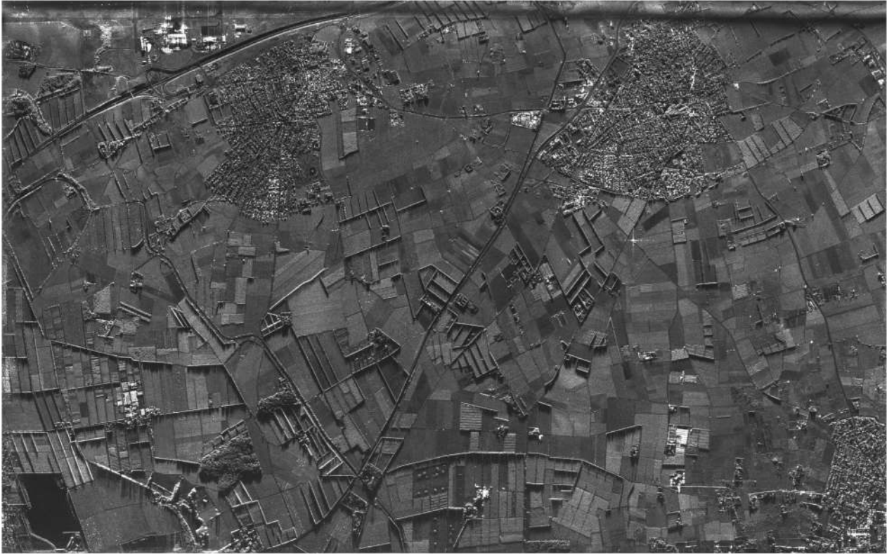
Fig. 10. BFFBP-processed bistatic image of one across-track configuration of DLR-ONERA airborne experiment. Radar illumination from top. Bistatic image is shown on highest resolution Cartesian grid. Increasing azimuth shown from left to right. Black stripe on top of image corresponds to elevation null of bistatic antenna pattern.
