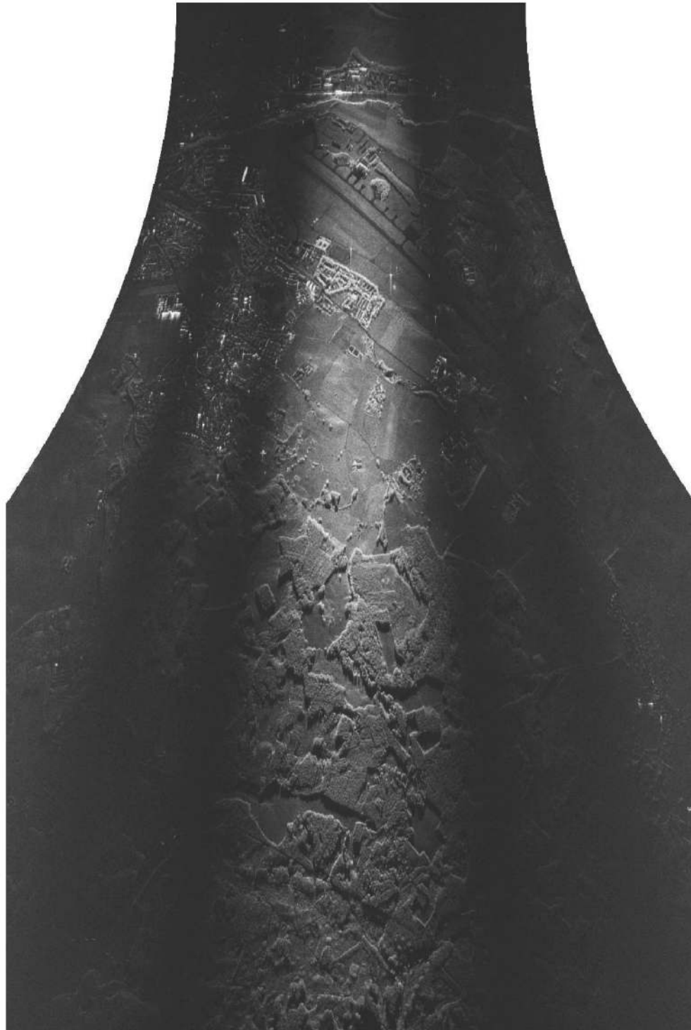
Fig. 8. BFFBP-processed bistatic image of TerraSAR-X/F-SAR first spaceborne-airborne experiment. Radar illumination from top. Bistatic image is shown on full-resolution elliptical grid, which causes slight curvature that can be observed. Low signal parts of image correspond to “nulls” of integrated bistatic azimuth antenna pattern.
