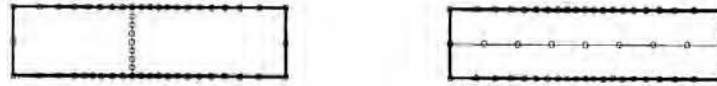
Figure 3. Influence of the splitting line length in the results. In the case on right, the centre of the domain will not be meshed with the proper density.
