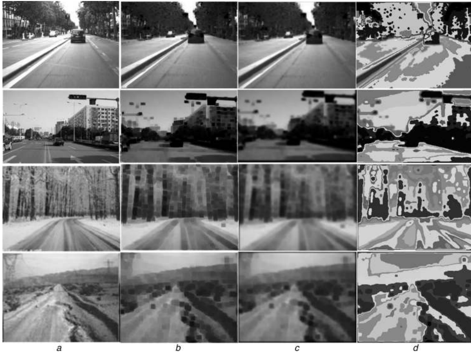
Fig. 2 Process of the image segmentation (a) Original image, (b) Dark channel prior image, (c) Dark channel image smoothed, (d) Segmentation results
