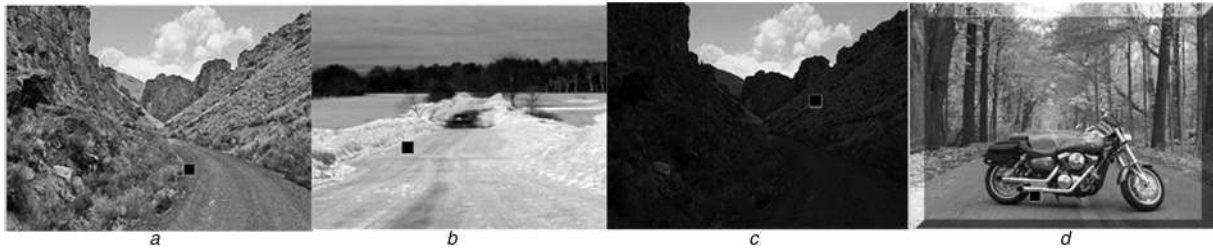
Fig. 10 Vanishing point detection results with large error (a) Vanishing point detection result on a mountain road image without obvious vertical lines, (b) Vanishing point detection result on a snow road image without obvious vertical lines, (c) Vanishing point detection result on a road image which has a small colour difference in the background and the road surface, (d) Vanishing point detection result on the road image with obstacles.
