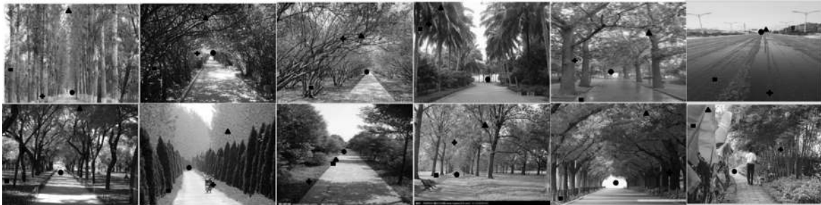
Fig. 9 Examples of road vanishing point detection results on road images with complex texture and background. The black points denote the detection results of our proposed method, the black squares are the detection results of Ding's method, the black triangles are the detection results of Kong's method and the black stars represent the detection results of gLoG method
