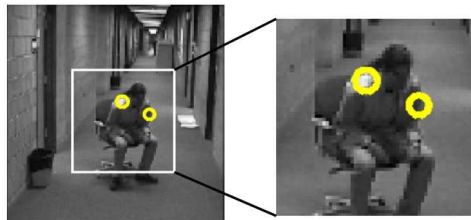
Figure 3: Space-time interest points are often found on highlights and shadows. These points are sensitive to lighting conditions and reduce recognition accuracy. This observation motivates our decision to apply volumetric features to the motion vectors rather than to the raw pixels.
