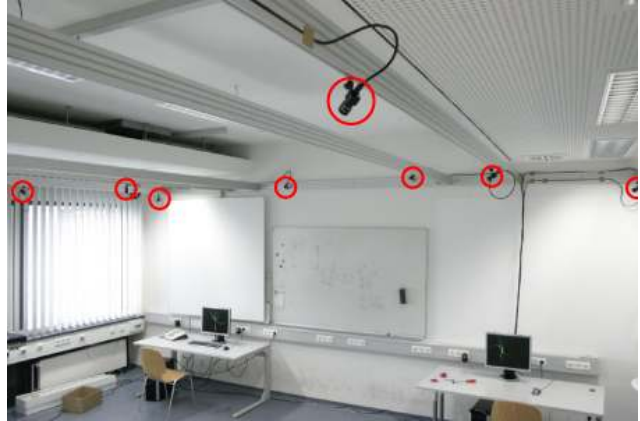
Figure 1. Lab setup for our real-time 3D reconstruction system. The cameras are marked with red circles (not all cameras are seen in this image).
