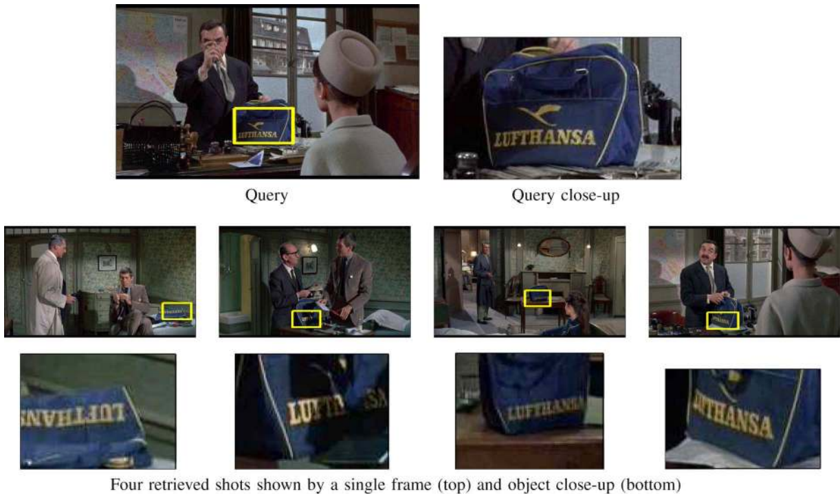
Fig. 1. Object query example I. Frames from top six ranked shots retrieved from a search of the movie “Charade” for visual query shown. Querying the entire movie took 0.84 s on a 2-GHz Pentium. A live demonstration of object retrieval system is available online [3].
