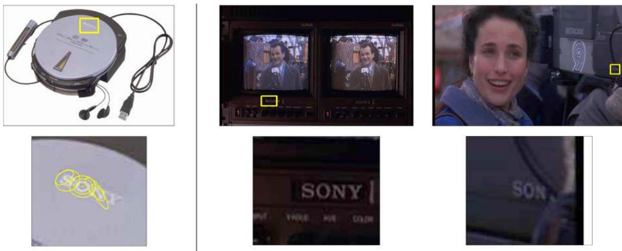
Fig. 15. Searching for a Sony logo. First column: (top) Sony Discman image ( 640 \times 422 pixels) with user outlined query region and (bottom) close-up with detected elliptical regions superimposed. Second and third column: (top) retrieved frames from two different shots of “Groundhog Day” with detected Sony logo outlined in yellow and (bottom) close-up of image. Retrieved shots were ranked 1 and 4.
