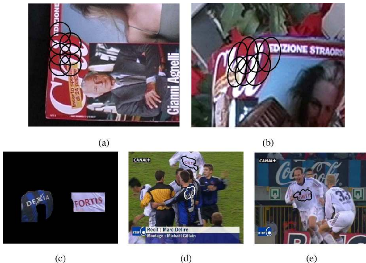
Fig. 18. (a), (b) Spatial verification based on overlap of local regions. (a) Set of local regions (shown in black) on a model view of object (magazine cover). (b) Same set of regions matched to a different view of same object. Note that pattern of intersection between neighboring regions is preserved despite the fact that object is imaged from a different viewpoint and deformed. (c), (e) Retrieval of deformable objects (logos on t-shirts) in video. (c) Two query objects delineated by user. Rest of the frame is blanked out. (d), (e) Examples of retrieved frames. Automatically found regions of interest are delineated in white and black. Figure courtesy of Ferrari, Tuytelaars, and Van Gool [15], [16].
