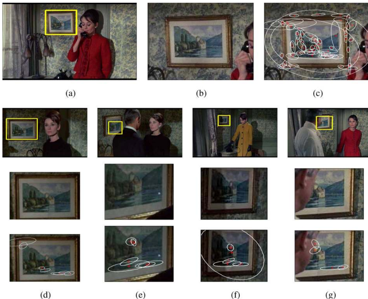
Fig. 11. Object query example IV: “Charade,” (a) Keyframe with user specified query region (a picture), (b) close-up of query region, and (c) close-up with affine covariant regions superimposed. (d)–(g) (First row) keyframes from 5th, 8th, 12th, and 18th retrieved shots with identified region of interest, (second row) close-up of image, and (third row) close-up of image with matched elliptical regions superimposed. First false positive is ranked 20th. Querying 6503 keyframes took 1.28 s on a 2-GHz Pentium.
