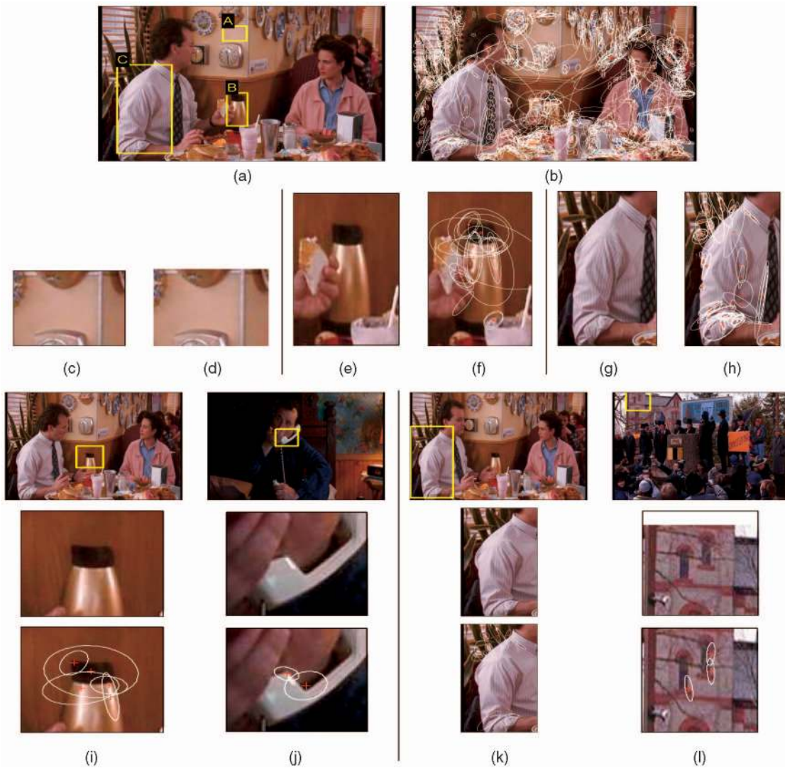
Fig. 15. Examples of challenging object searches. (a) Keyframe from the movie “Groundhog Day” with three query regions (denoted as A, B, and C). (b) The same keyframe with affine covariant regions superimposed. (c), (e), and (g) Query region close-ups. (d), (f), and (h) Query close-ups with affine covariant regions superimposed. (i)-(l) Example retrievals for (i)-(j) object B and (k)-(l) object C. Each column shows (top) a keyframe from the retrieved shot with the identified region of interest, (middle) a close-up of the image, and (bottom) a close-up of the image with matched affine regions superimposed. Query analysis: Query A (plain wall) does not contain any visual words and hence returns no results. Query B (coffee pot) retrieves two shots taken from very similar viewpoints (the second ranked is shown in (i)). Other shots are not retrieved as affine regions extracted on the object either include background or cover specular reflections, which change with viewpoint and lighting conditions. The first false positive (ranked third) is shown in (j). Query C (the white shirt) retrieves three correct shots (the second ranked is shown in (k)), but most of the matches are on the background object. This is because affine regions on the shirt are detected on creases, which change as the person moves. The first false positive (ranked fourth) is shown in (l).
