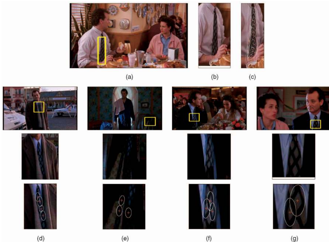
Fig. 11. Object query example 5: Groundhog Day. (a) Keyframe with user specified query region (tie), (b) close-up of the query region, and (c) close-up with affine covariant regions superimposed. (d)-(g) (first row) Keyframes from the 1st, 2nd, 4th, and 19th retrieved shots with the identified region of interest, (second row) a close-up of the image, and (third row) a close-up of the image with matched elliptical regions superimposed. The first false positive is ranked 25th. Querying 5,640 keyframes took 0.38 second on a 2 GHz Pentium.
