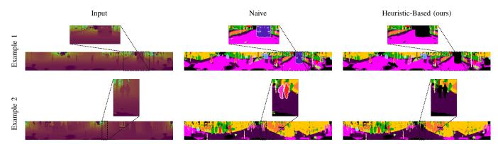
Fig. 8: Comparison of pseudo labels generated naively and using our proposed heuristic. On the left, the full range image is shown with zoomed in regions. Each example shows the predictions of the full image with zoomed in regions and the input range image. The labels generated using the naive heuristic misclassifies the truck (purple) in example 1 and a person as bicyclist (light purple) in example 2. Our proposed heuristic assigns the misclassified pixels as unlabeled in both examples.
