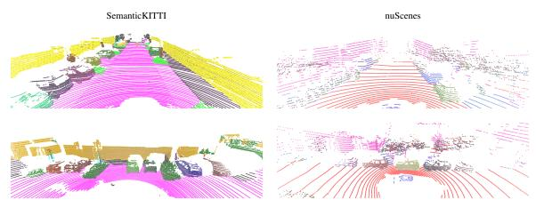
Fig. 5: Example groundtruth visualization from SemanticKITTI and nuScenes datasets. The SemanticKITTI dataset was collected using a 64-beam LiDAR, hence it provides a fairly dense representation of the environment in comparison to the nuScenes dataset which was collected using a 32-beam LiDAR.
