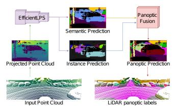
**Fig. 1:** Overview of the top-down EfficientLPS architecture that consists of a shared backbone to learn spatially-aware features from the projected point cloud and individual heads to learn semantic and instance specific features which are fused in the panoptic fusion module. The network explicitly utilizes the range information in the backbone, semantic head and fusion module to mitigate the problems due to the projection and distance-dependent sparsity of LiDAR point clouds.
