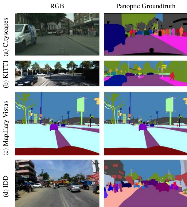
Fig. 5 Example images from the challenging urban scene understanding datasets that we benchmark on, namely, Cityscapes, KITTI, Mapillary Vistas, and Indian Driving Dataset (IDD). The images show cluttered urban scenes with many dynamic objects, occluded objects, perpetual snowy conditions and unstructured environments
