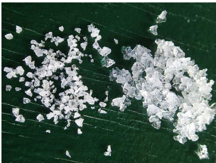
Figure 1. Hydrogel crystals before (left) and after (right) saturation with a sucrose (25%) solution. Twenty grams of dry crystals expands to make approximately one liter of bait.
