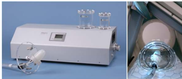
Fig. 1 The dynamic heart phantom. Left —the membrane and pump units. Right —the phantom assembled and ready for measurement in the gamma camera. The membrane unit installed is shown inside a NEMA IEC PET body phantom and positioned for IQ-SPECT acquisition
