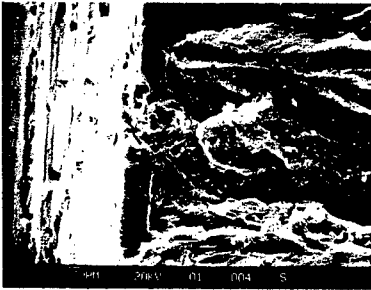
Figure 9 SEM-micrograph of the crack area with striations – bell S
